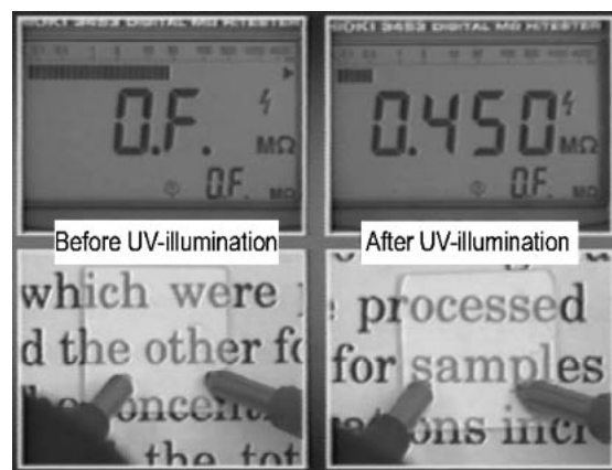
Fig. 17. Conversion from insulating to conductive states in an H^- -incorporated C12A7 thin film (thickness: 200 nm) by ultraviolet light illumination. The color and the transparency of the film remains unchanged after by the conversion.
